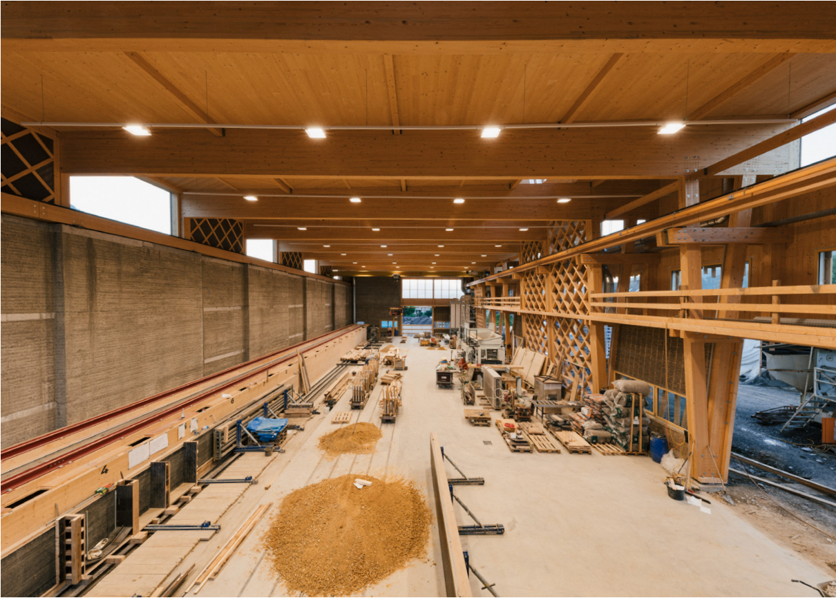
10 ERDEN factory workshop for prefabricating rammed earth elements
