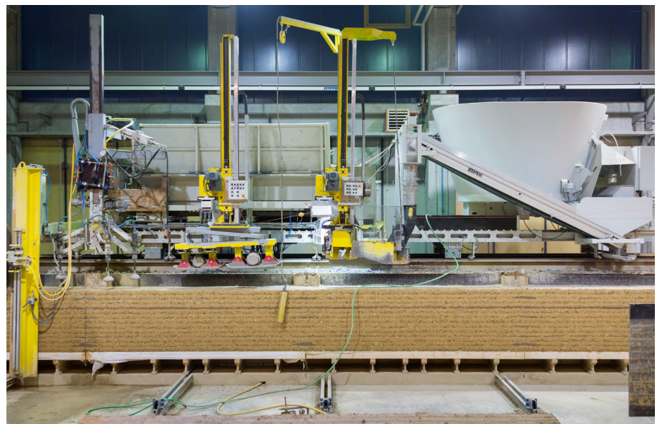
04 "Roberta" – a machine for the production of prefabricated rammed earth elements
