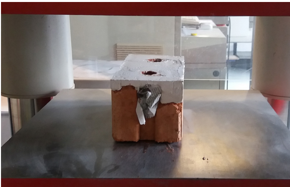
17+18 Compressive strength testing at the Kompetenzzentrum Bau MV (Wismar University of Applied Sciences)
