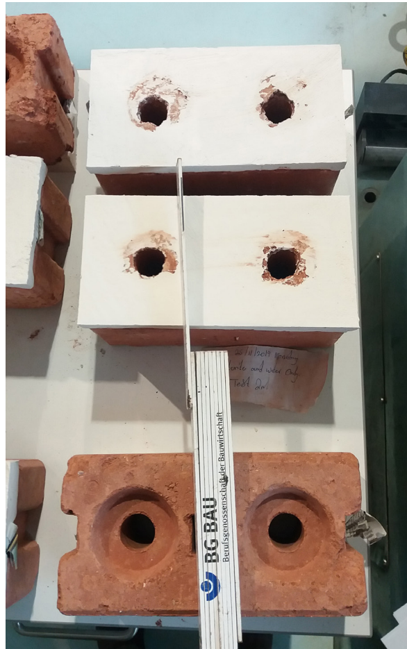
17+18 Compressive strength testing at the Kompetenzzentrum Bau MV (Wismar University of Applied Sciences)
