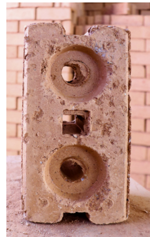
05-07 The special feature of MAGGLO bricks are their interlocking forms that can be assembled without mortar
