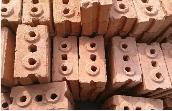
03+04 Unfired, compressed bricks made of red laterite earth with smooth surfaces
