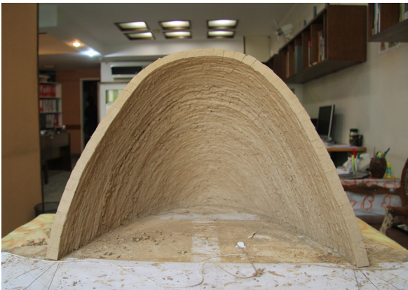
15 We made a prototype of the structure in different site, in order to analyze it and become more familiar with its challenges. ©Sonia Beygi
