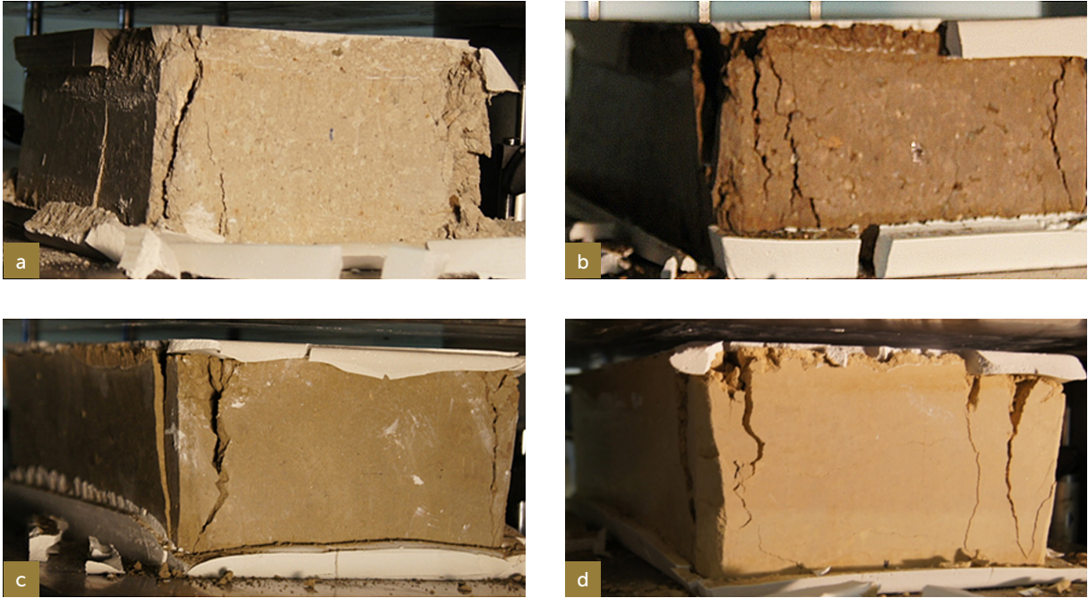
03 Compression failure mode of CEB units made of (a) A-soil, (b) D-soil, (c) T-soil and (d) L-soil
